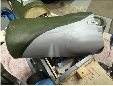
I'm quite happy with how she turned out. The battery hatch on top took some head scratching - especially on the double latch set up. The motor and ESC were relatively easy to place. I am concerned about whether I have enough air flow for cooling though with just a hole at the bottom of the cowl and venting out the exhaust stacks. The motor is an e-Flite Power 60 and 80 amp ESC. A 6-cell 4,000 battery fits nicely in the battery compartment.
